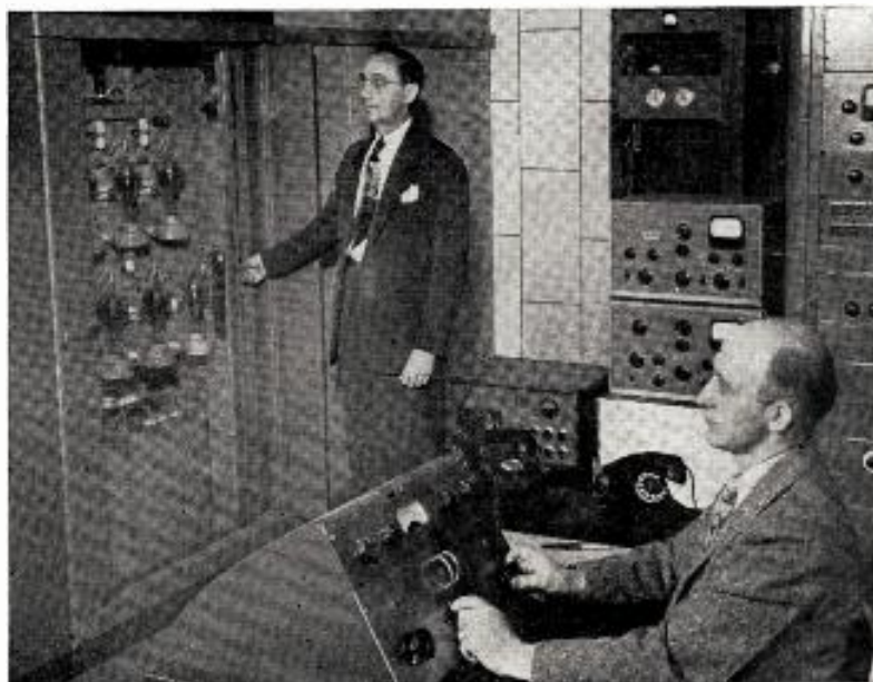
MANIPULATING the switch, Arthur F. Rekart (l), chief engineer, turns on the KXOK-FM St. Louis new 10 kw transmitter located in the Boatmen's Bank Bldg. in downtown St. Louis. Robert V. Nicholas, assistant, operates the control panel. New facilities, in operation since April 27, enable the station to broadcast with a radiated power of 70 kw in a 17,500 square mile area. Its new tower rises 574 ft. above street level. KXOK-FM, affiliated with Transit Radio Inc., broadcasts continuous music-news-weather programs to 1,000 buses and streetcars of the St. Louis Public Service Co.
